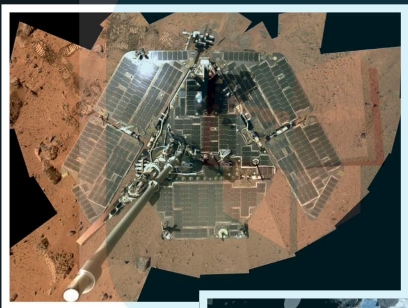
This top view of the Mars Exploration Rover Spirit (a self-portrait) shows solar panels coated in reddish Mars dust. Flip to Chapter 3 to see how solar panels power spacecraft.
